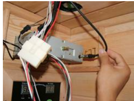
FIG-20 Link the antenna connectors
