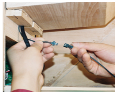
FIG-18 Link the sensor connectors
