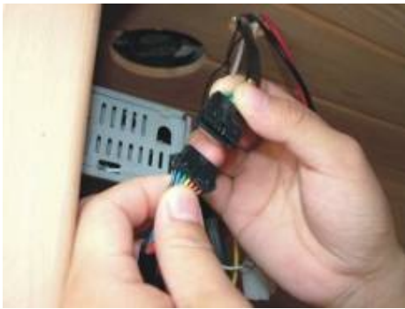
FIG-19 Link the control panel connectors
