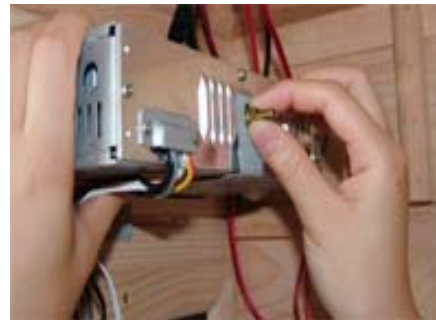
FIG-16.3 Lock the CD with its metal support
