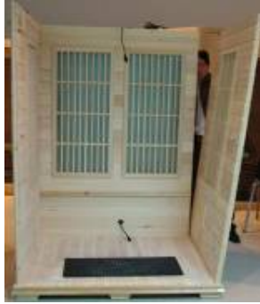
FIG-7 Assembling right board
