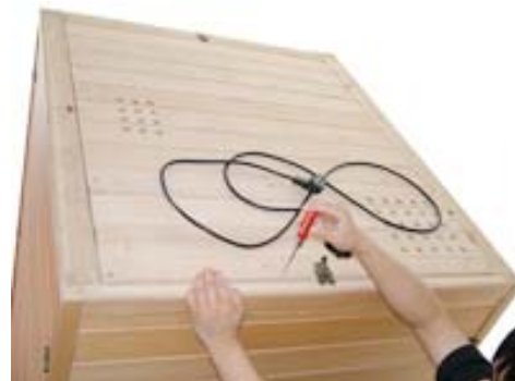
FIG-23 Fix the external board with screws
